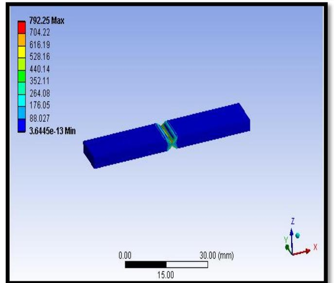
**Fig.20.** Heat Flux on the welded pieces.
