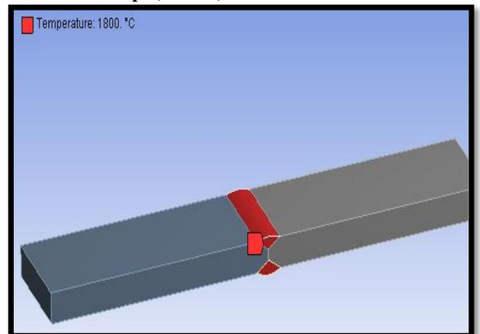
**Fig.21.** Temperature is applied at the welded region.
