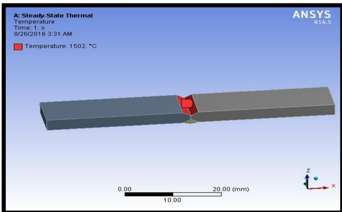
**Fig.15. Temperature is applied at the welded region.**
