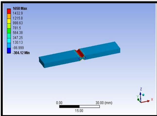
**Fig.19.**Temperature distribution on the welded pieces.
