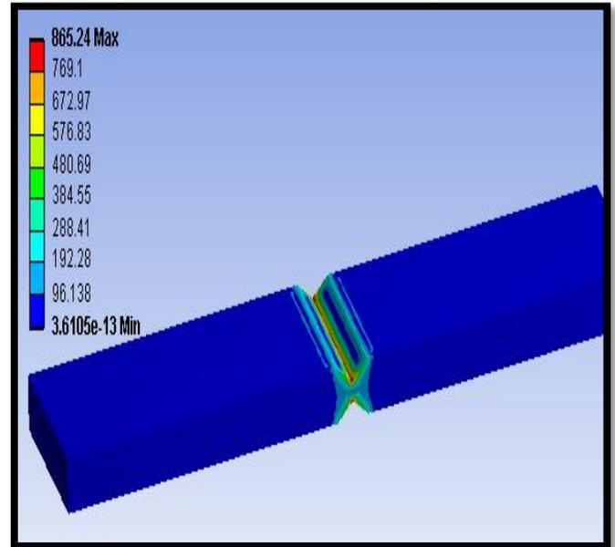
Fig.23. Heat Flux on the welded pieces.
