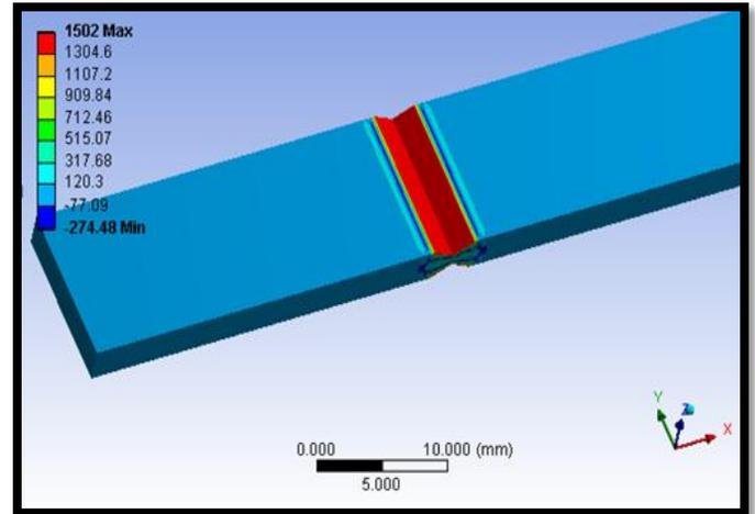
**Fig.16. Temperature distribution on the welded pieces.**
