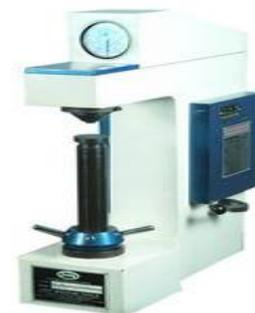
Fig.11. Brinell/Rockwell hardness tester.
