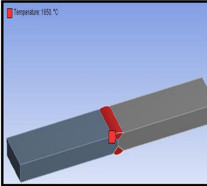
**Fig.18.**Applied Temperature at the welded region.
