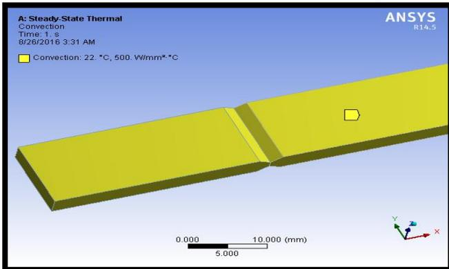
**Fig.14. Applying of convection.**
