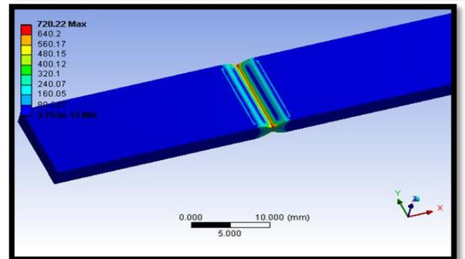
**Fig.17. Heat Flux on the welded pieces.**
