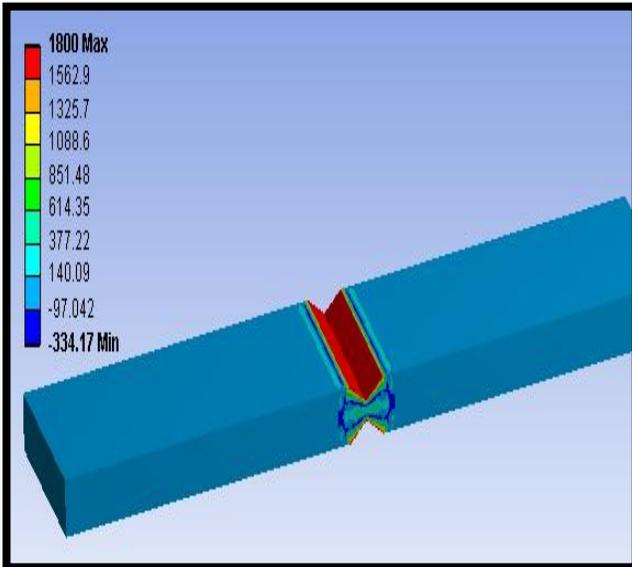
Fig.22. Temperature distribution on the welded pieces.
