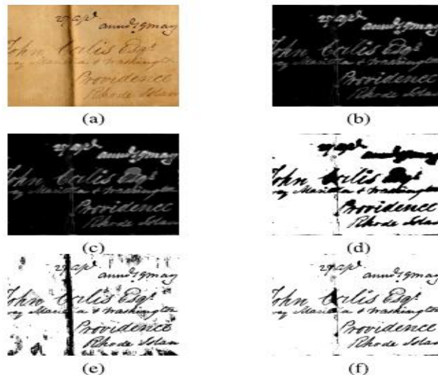
Fig. 5. A degraded document image and its binarized image using phase congruency. a) Original degraded document image. b) Edge image obtained by phase congruency (IM). c) Filled image of IM. d) Binarization of (c) using Otsu's method. e) Denoised image and f) The result of main binarization.
