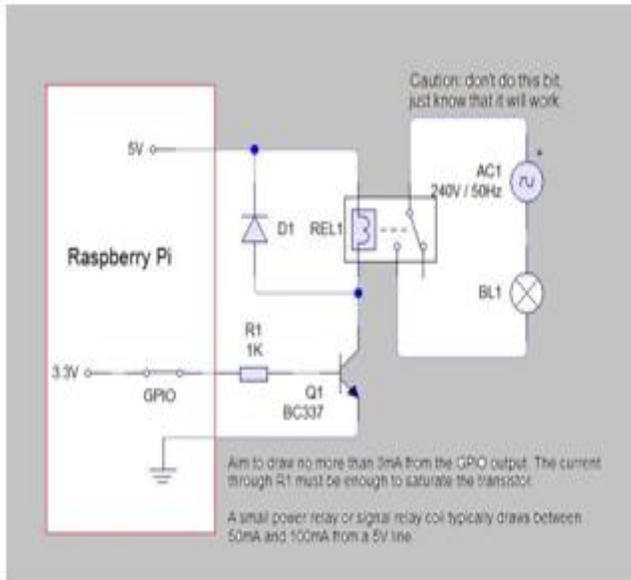
Fig.7. Relay connected with raspberry-pi.
