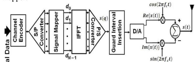
Fig.1. A typical OFDM transmitter.
