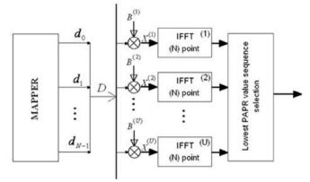
Fig. 2. Conventional SLM technique at the transmitter end.
