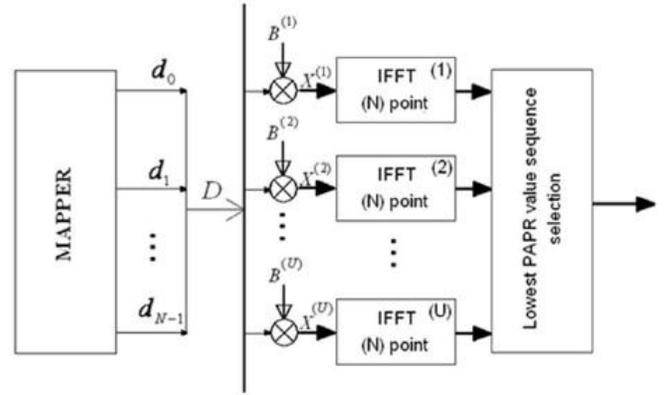
Fig. 2. Conventional SLM technique at the transmitter end.
