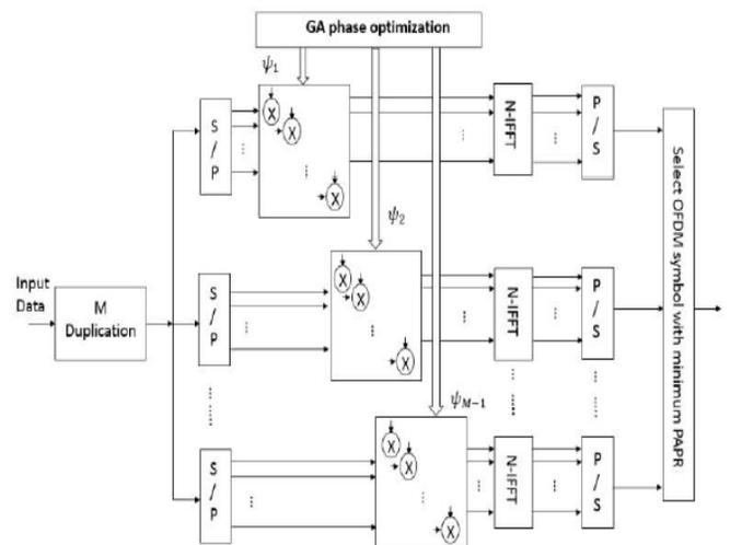
Fig.3. Functional block diagram of the proposed GA based SLM-OFDM technique.
