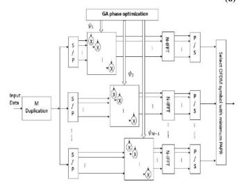
Fig.3. Functional block diagram of the proposed GA based SLMOFDM technique.
