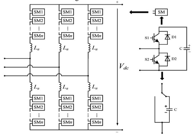
**Fig. 2. Structure of one MMC and a SM.**
