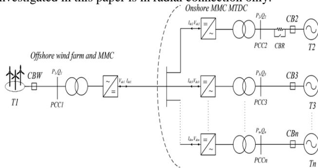
**Fig. 1. MMC MTDC system with the integration of an OWF.**
