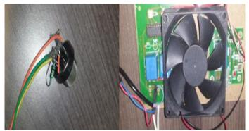
Fig.2.MQ2 Gas sensor and Exhaust Fan.
