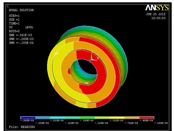
Fig.16. Displacement of Bearing.
