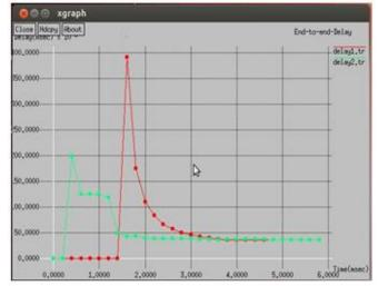
The delay between source to destination is less. AODV has the information of the routes which are active and thus when
