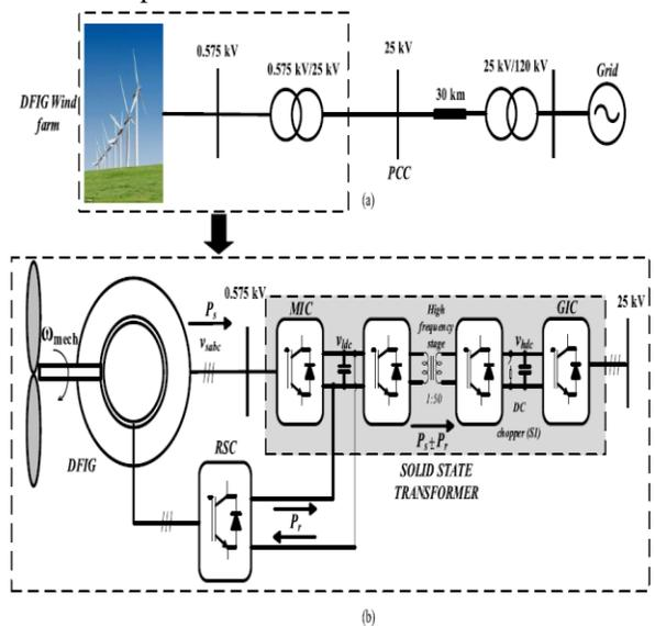
**Fig.2. (a) Regular DFIG configuration and (b) Proposed SST based DFIG configuration.**
