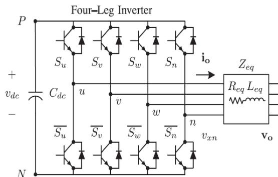
Fig. 2. VSI connected to grid using DC capacitor.
