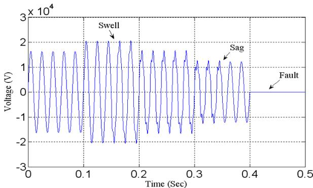
Fig. 3. Voltage profile with sag, swell & harmonics.
