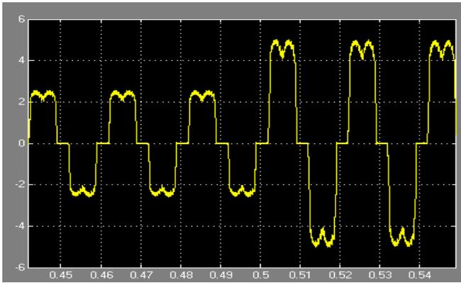
Fig. 8. Load current of Phase A.
