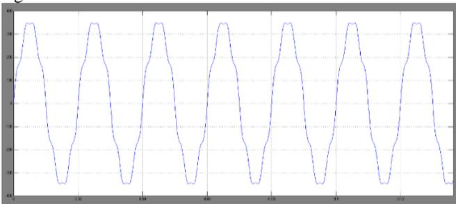
**Fig.6. Current in the grid winding of the new grid-connected transformer without inductive filtering method.**
