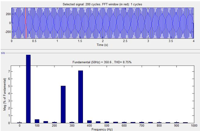
**Fig.7. FFT results on the current waveform in the without filter.**
