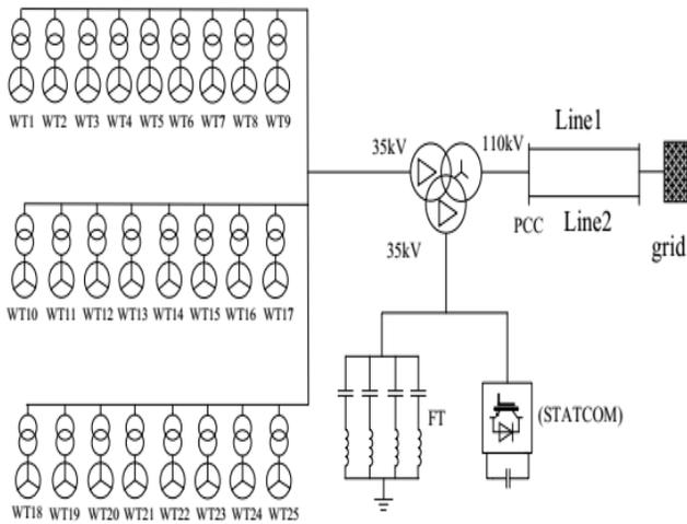
Fig.1. Main circuit topology of the grid connected wind power system.
