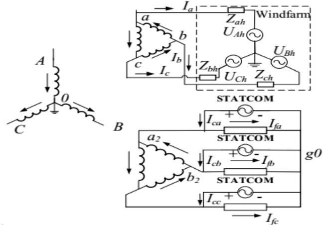
Fig. 3. The current distribution of the new grid connected transformer.
