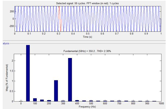
**Fig.9. FFT results on the current waveform in the with filter.**
