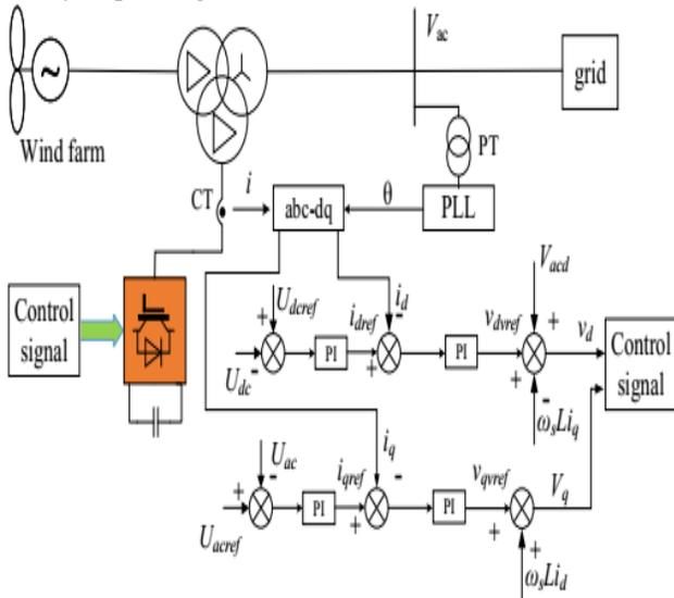
**Fig.5. Schematic diagram of STATCOM controller.**
