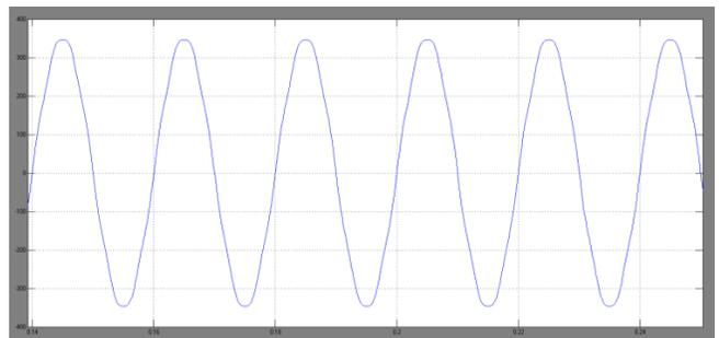
**Fig.8. Current in the grid winding of the new grid-connected transformer with inductive filtering method.**
