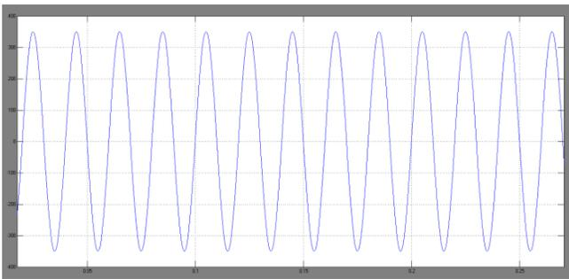
Fig.15.phase to phase voltage of inverter.
