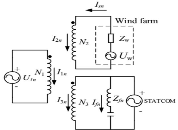
Fig.2. the single-phase equivalent-circuit model of the new grid connected transformer with FT branches.
