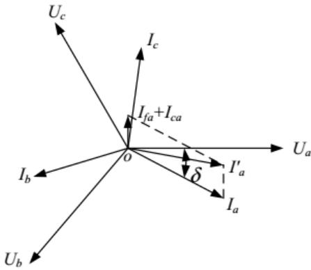
**Fig.4 Phasor diagram of the voltage and current of the secondary winding.**
