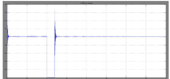
**Fig. 11. Magnitudes of the voltage at the PCC with STATCOM.**
