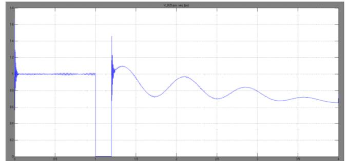
**Fig. 10. Magnitudes of the voltage at the PCC without STATCOM.**
