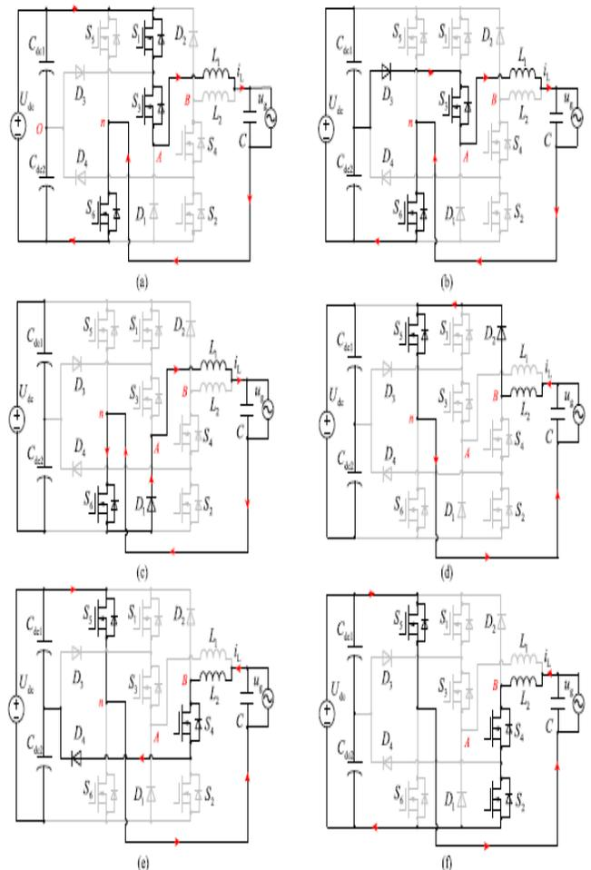
Fig4. Equivalent circuits of switching state, (a) State #1. (b) State #2. (c) State #3. (d) State #4. (e) State #5. (f) State #6.
