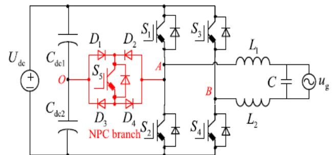
**Fig2. Simplified five-level H-bridge inverter topology.**
