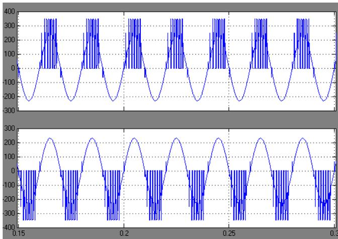
**Fig7.** Simulation waveforms of the SS five-level DBFBI.  $u_{An}$  and  $u_{Bn}$ .
