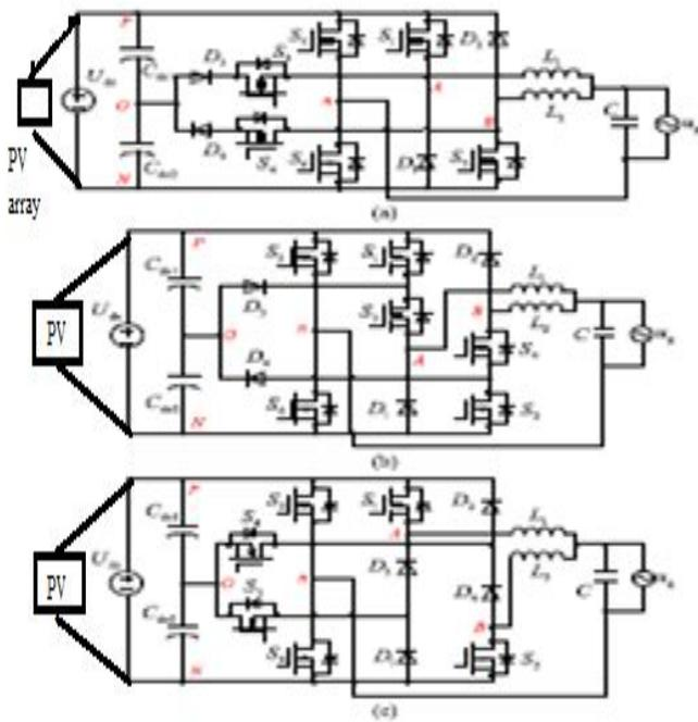
Fig3. Three topologies of five-level DBFBIs proposed, (a) NPC fivelevel DBFBI. (b) Series-switch five-level DBFBI. (c) Series-diode five-level DBFBI.
