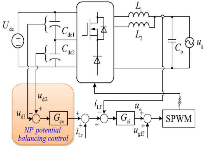
**Fig. 6.** Control block of five-level DBFBIs.
