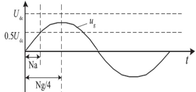
**Fig5. Sketch diagram of the switching times.**
