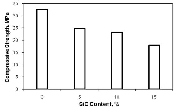
Fig.44. Compressive strength v/s wt% of SiC.
