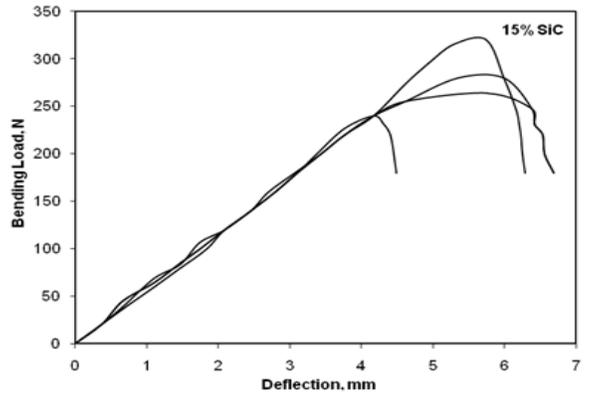
Fig.34. load v/s deflection graph for 15% SiC filled specimens.
