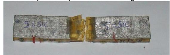
Fig.46. Fractured compression test specimen.
