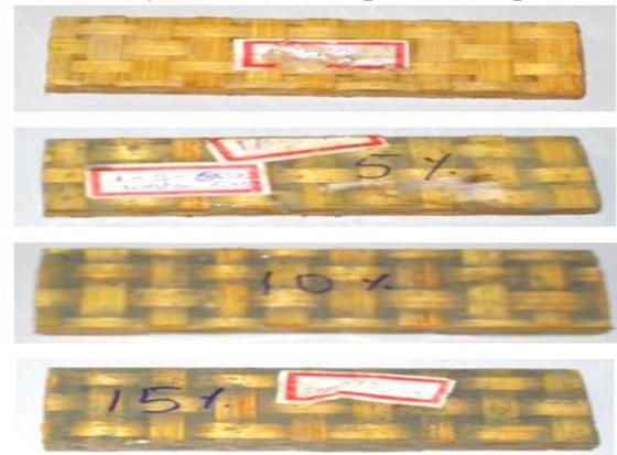
**Fig.17. Water Absorption Test Specimens.**
