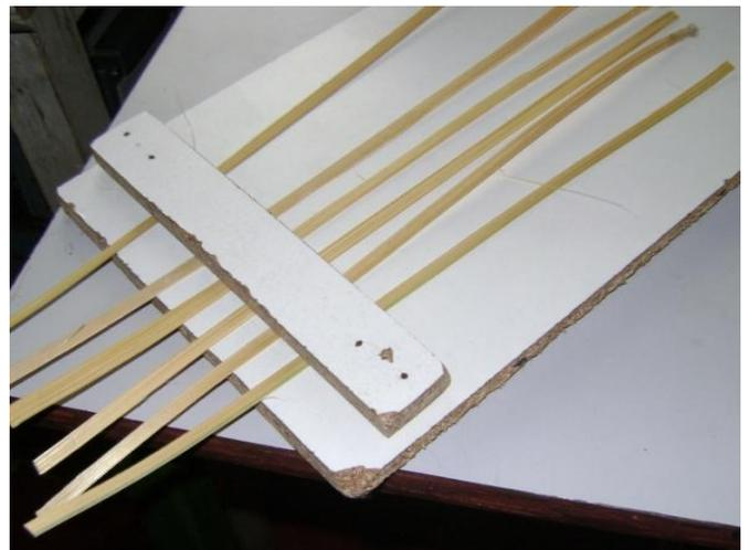
Fig.3. Measuring thickness of bamboo strips using go-gauge.
