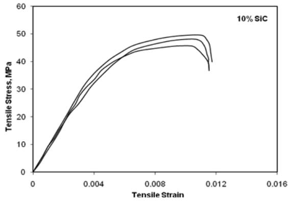
Fig.24. stress v/s strain graph for 10% SiC filled specimens.
