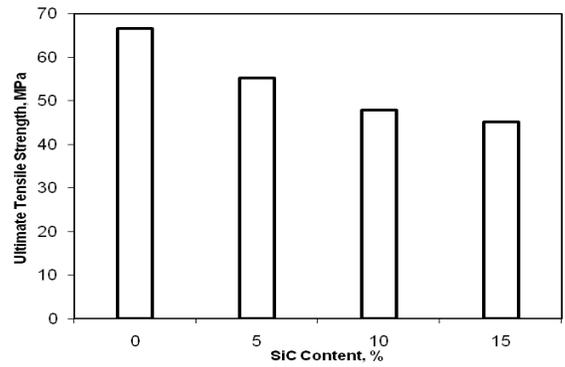
Fig.27. Tensile strength v/s wt% of SiC.
