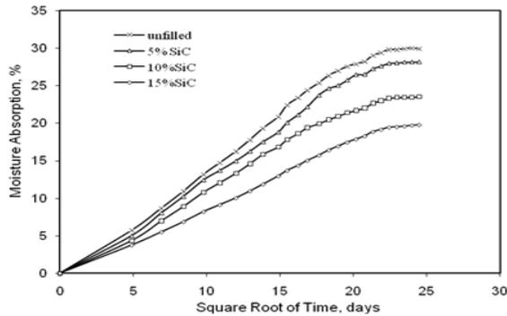
**Fig.47. Moisture Absorption v/s Square root of time Graph for Different combinations.**
