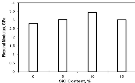
**Fig.37. Flexural Modulus v/s wt% of SiC.**
