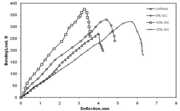
Fig.35. Bending Load v/s Deflection Graph for Different combinations.
