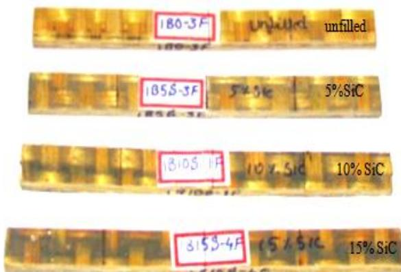
**Fig.13. Flexural Test Specimens.**
