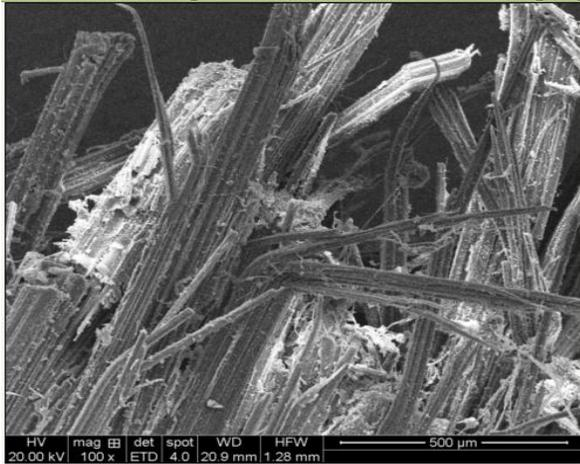
Fig.52. SEM image of Unfilled Tension tested specimen.
