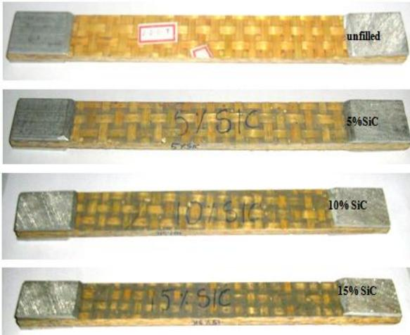
**Fig.11. Tension Test Specimens.**
