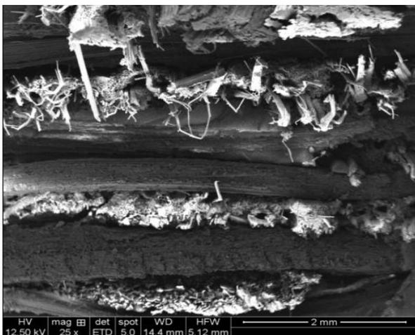
Fig.54. SEM image of Unfilled Flexural tested specimen.
