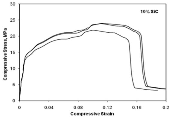
Fig.41. Stress-Strain Graph for 10% SiC filled composites.
