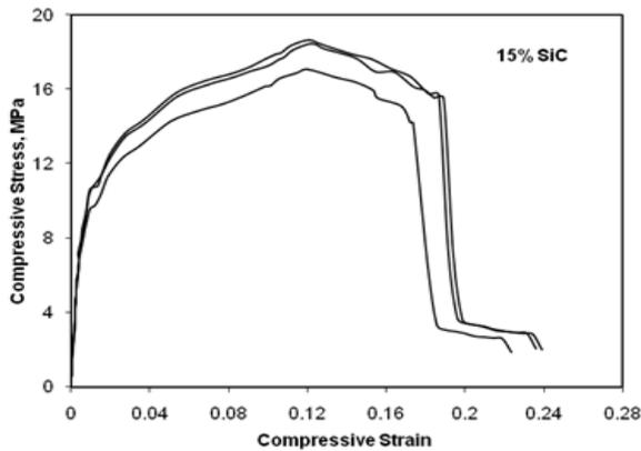
Fig.42. Stress-Strain Graph for 15% SiC filled composites.
