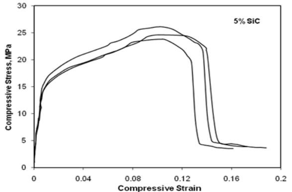
**Fig.40. Stress-Strain Graph for 5% SiC filled composites.**
