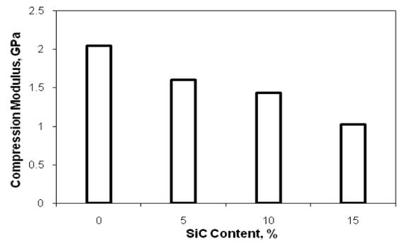
Fig.45. Compression Modulus v/s wt% of SiC.
