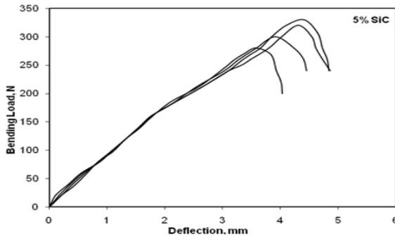
Fig.32. load v/s deflection graph for 5% SiC filled specimens.
