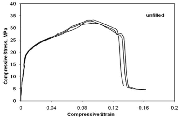
**Fig.39. Stress-strain graph for unfilled composites.**
