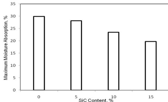
**Fig.49. Moisture Absorption v/s wt % of SiC.**
