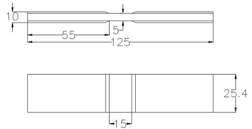
**Fig.14. Geometry of Compression Test Specimen.**
