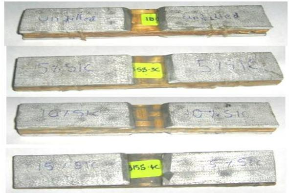
**Fig.15. Compression Test Specimens.**
