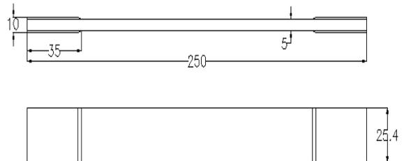
Fig.10.Geometry of Tensile Test Specimen.
