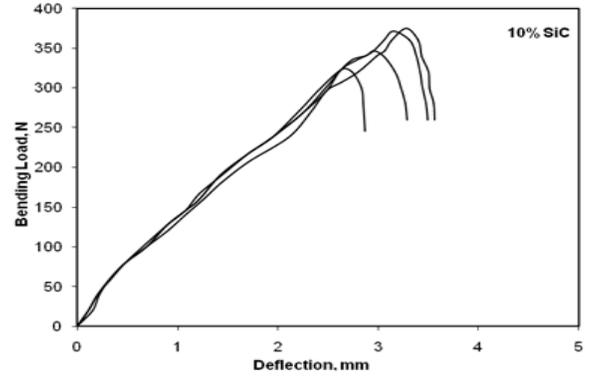
Fig.33. load v/s deflection graph for 10% SiC filled specimens.
