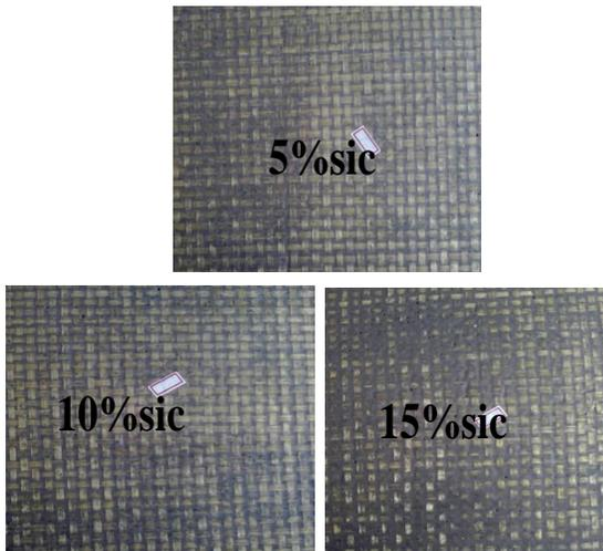
Fig.9. 5, 10, 15% SiC filled (with respect to wt% of epoxy) bamboo laminates.
