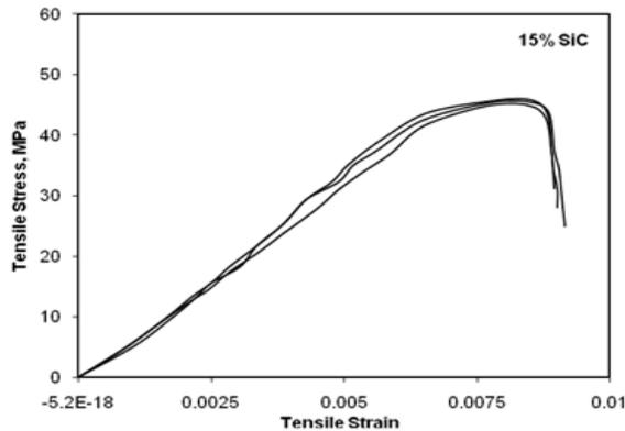
Fig.25. stress v/s strain graph for 15% SiC filled specimens.
