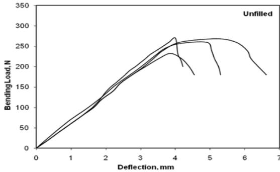
Fig.31. load v/s deflection graph for unfilled specimens.
