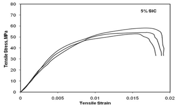
Fig.23. stress v/s strain graph for 5% SiC filled specimens.
