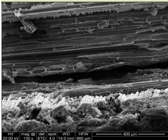
Fig.53. SEM image of 10%SiC filled Tension tested specimen.
