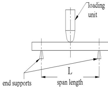
**Fig.12. Geometry of Flexural Test Specimen.**
