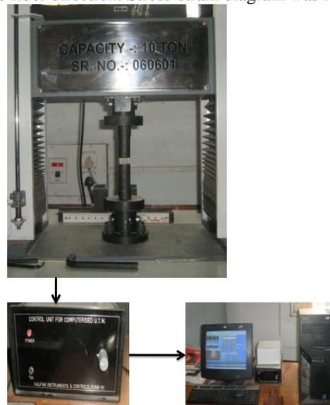
**Fig.20. compression test setup.**
