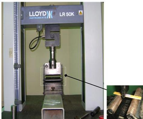
**Fig.19. Flexural test setup.**
