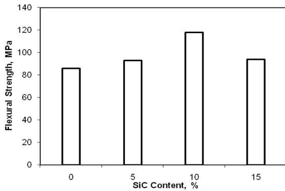
**Fig.36. Flexural strength v/s wt% of SiC.**
