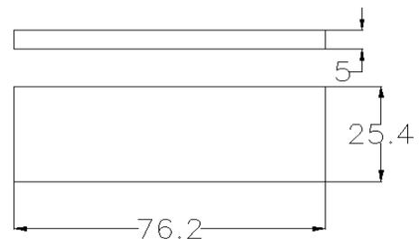
**Fig.16. Geometry of Water Absorption Test Specimens.**
