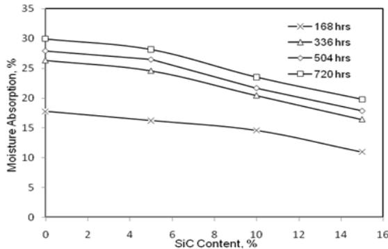
**Fig.48. Moisture Absorption v/s SiC content Graph for Different time.**
