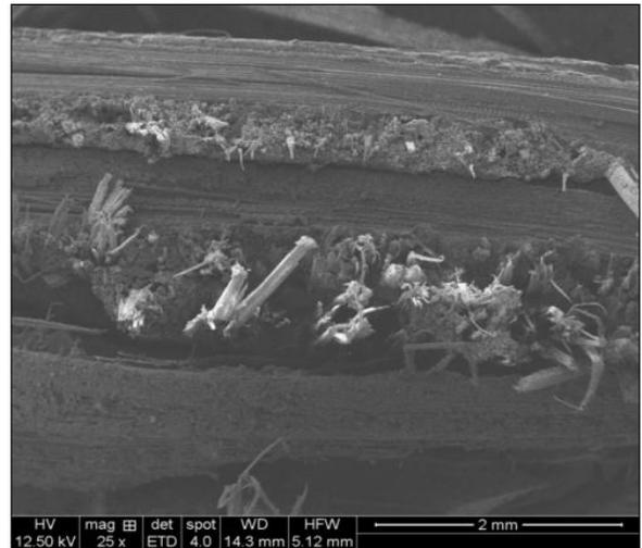
Fig.55. SEM image of 10%SiC filled Flexural tested specimen.
