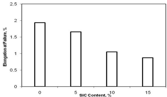
Fig.29. Percentage Elongation at Failure v/s wt% of SiC.
