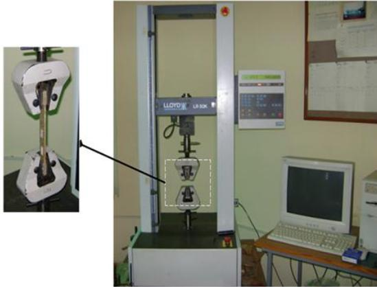
**Fig.18. Tensile test setup.**
