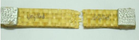
Fig.30. Fractured tension test specimen.
