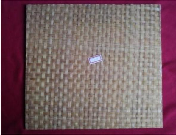
Fig.8. unfilled bamboo laminate
