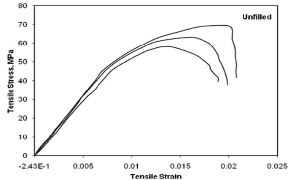
Fig.22. stress v/s strain graph for unfilled specimens .
