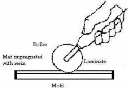
Fig.5. Hand Lay-Up technique.
