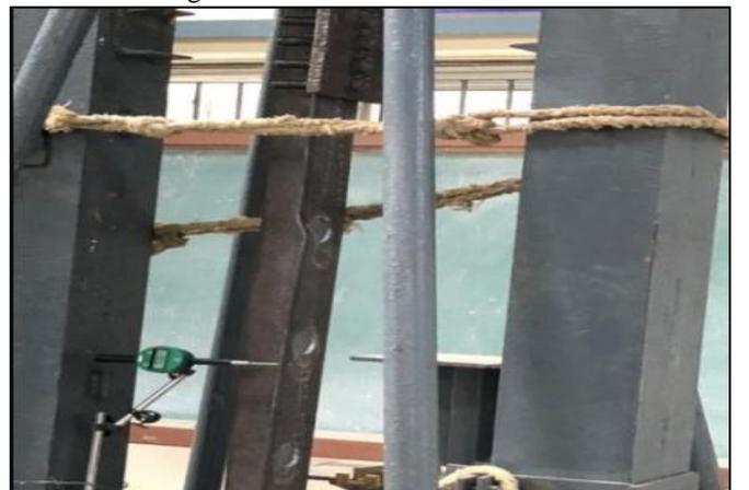
Fig.34. Deflected shape for loaded leg perforated member.
