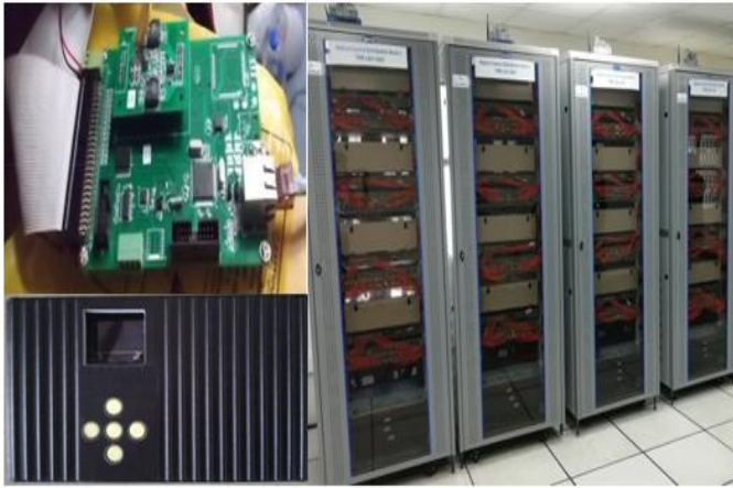
Fig2.The ARM cortex-m4 unit interface of radar transmitters.
