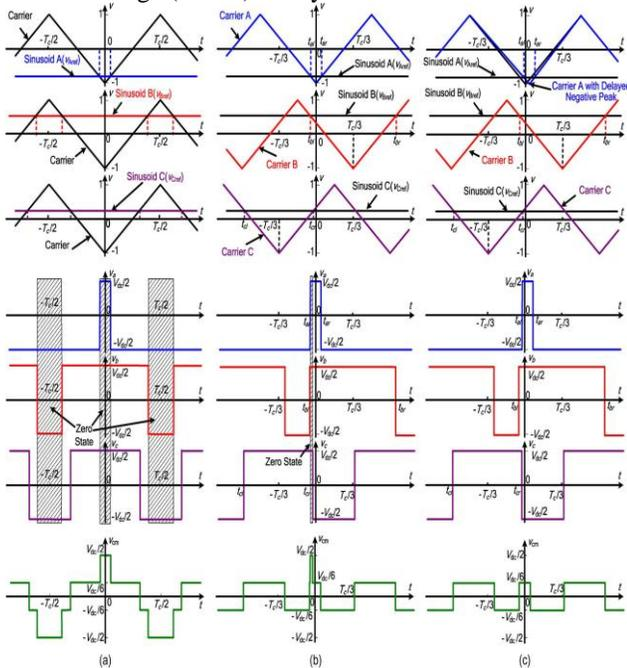
**Fig. 6. Modulation of three-phase reference voltages with different carriers (top), three-phase output pulses (middle) and output CMVs (bottom) in the three-phase inverter under (a) the conventional SPWM strategy, (b) the CPS strategy, and (c) the CPPM strategy.**
