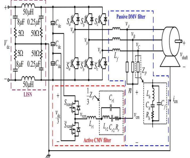
**Fig. 7. Three-phase inverter with the hybrid filter.**
