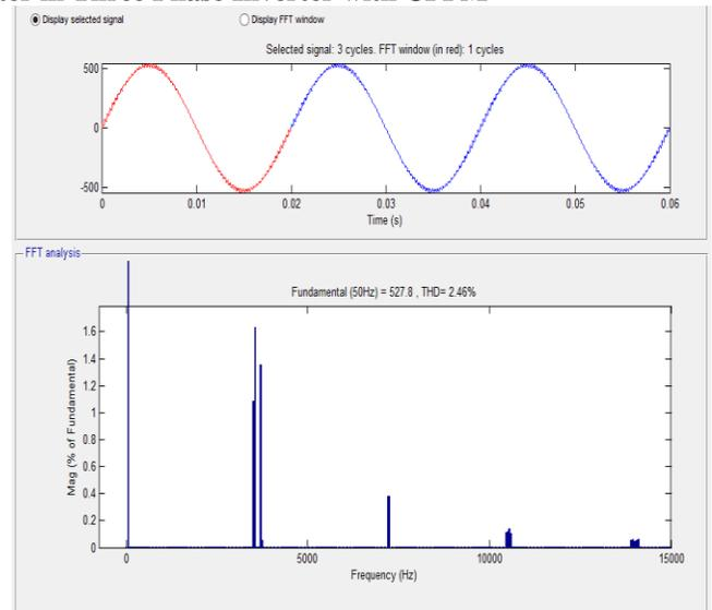
**Fig.10 (c).** THD of DM harmonics under CPPM with a Hybrid filter.
