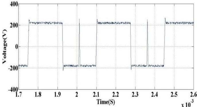
Fig.8 (b). CMV in three-phase inverter under the CPPM strategy without Hybrid filter.
