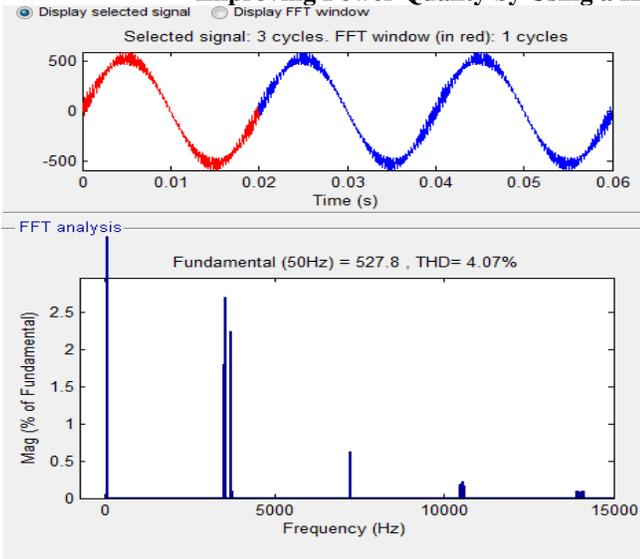
**Fig.10(a).** THD of DM harmonics under SPWM strategy without Hybrid filter.
