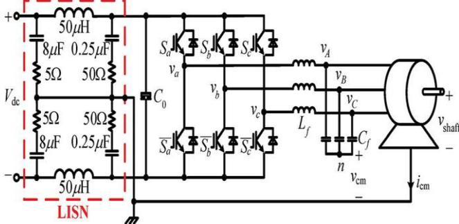
**Fig. 5. Three-phase inverter.**
