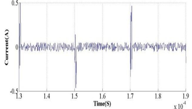
Fig.9(a). CMC in the three-phase inverter under SPWM strategy without Hybrid filter.
