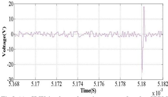
Fig.8 (c). CMV in three-phase inverter under the CPPM strategy with Hybrid filter.
