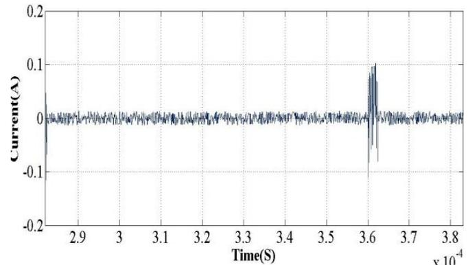
Fig.9(c). CMC in the three-phase inverter under the CPPM strategy with Hybrid filter.
