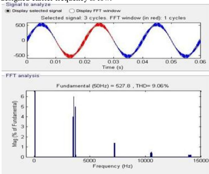
**Fig.10 (b).** THD of DM harmonics under CPPM strategy without Hybrid filter.
