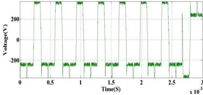
Fig.8 (a). CMV in three-phase inverter under the SPWM strategy without Hybrid filter.
