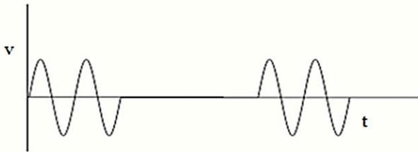
**Fig.1. Voltage Signal with Long Interruption.**
