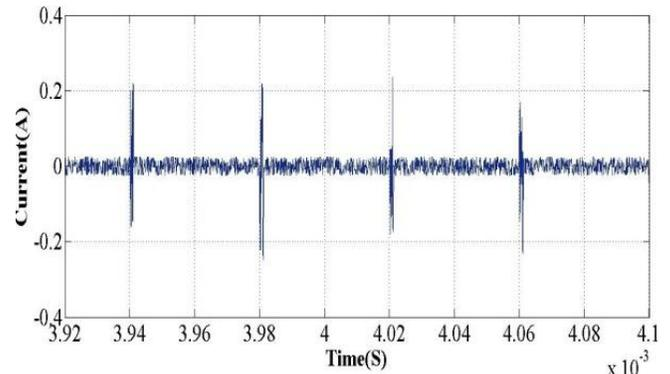
Fig.9(b). CMC in the three-phase inverter under CPPM strategy without Hybrid filter.
